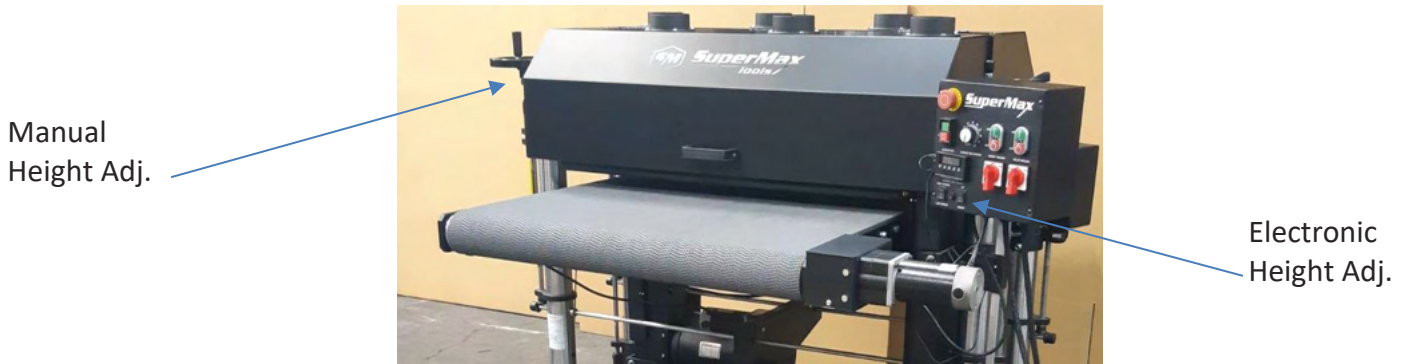
Figure 16: Height Control Adjustments
