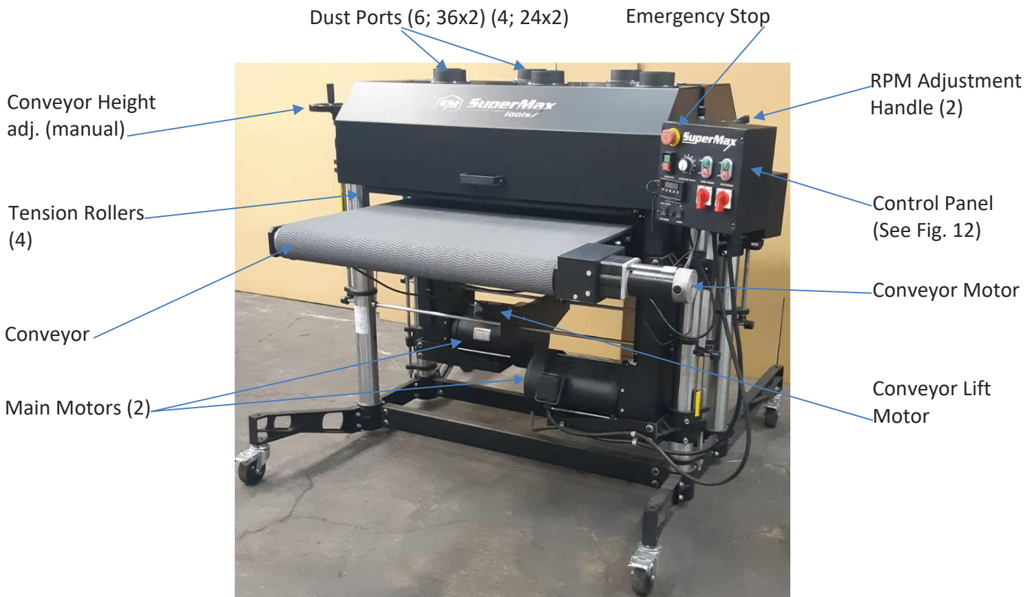
Figure 10: Main Components of SuperBrush 36 x 2 (similar to SB 24 x 2)
