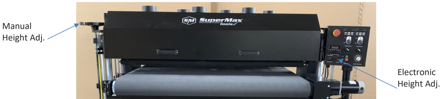
Figure 16: Height Control Adjustments
