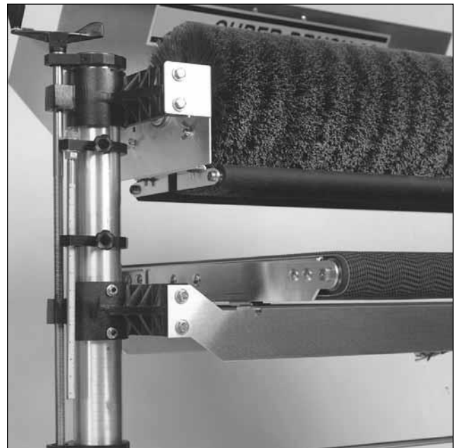
Fig. 16. Height controls on outboard side.
