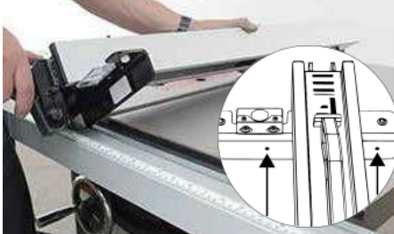
Position fence to access adj. screws
