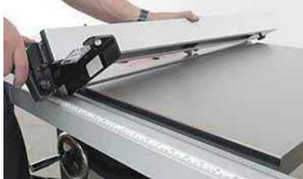
2. Place fence in fence guide
