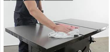
Wipe off protective plastics
