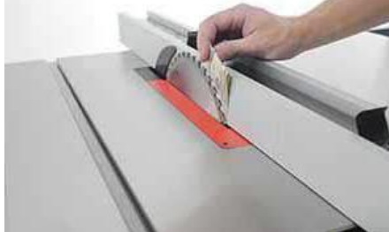
Place fence in fence guide
