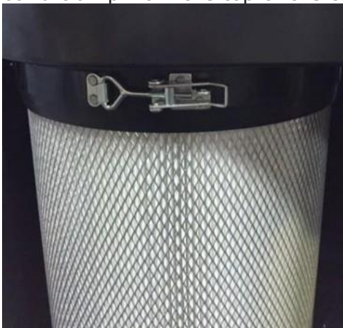
Figure 8: Hold canister from bottom when releasing clamp
