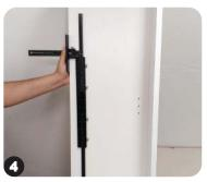
Slide Extended Ruler Attachment into Extension Bar, align any drill bushing with mark in cabinet from Step 1, tighten Thumb Screws.
