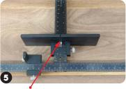
Set Large Stop to measurement from Step 4 and tighten.
