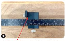
Set Sliding End Stop on Extended Ruler at half the measurement from Step 1.
