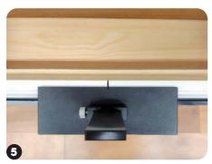
Line up notch on center of Large Stop with center mark at top of drawer then push tool flush against drawer face.
