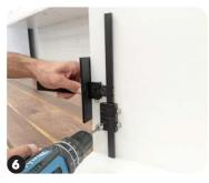
Flip tool to bottom of cabinet, position tool with Large Stop and T-Square firmly against cabinet surface, and drill second set of holes.
