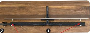
Match the bottom hole on hardware to bottom hole on Extension Bar and mark with tape.
