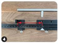
Attach Extended Ruler and set at index mark for bottom hole. Set Sliding End Stop to measurement from Step 2.
