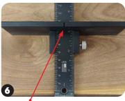
Set Large Stop to half of measurement from Step 5 (if centering).
