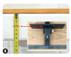
Measure height of drawer and set Large Stop to desired location and tighten Thumb Screws (half of measurement, if centering).
