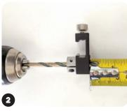
Set Depth Stop Collar to drill depth and tighten. Depth varies depending on screw type and cabinet material.
