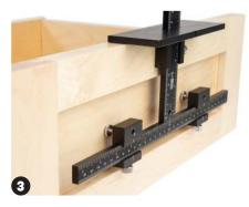
Return Sliding Drill Guides to appropriate measurements to install cabinet hardware.
