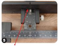
Set Large Stop to measurement from Step 4 and tighten.
