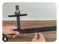
Slide the Extension Bars all the way onto the T-Square, and tighten all four Thumb Screws.
