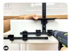
For Handles: Measure hardware and tighten Sliding Drill Guides to match hardware measurement then drill (refer to Page 6, Handle on Drawer section if more information is needed).
