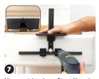
Line up notch on Large Stop with mark from Step 4, then drill.
