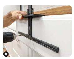
Hold securly and drill hole using fixed center drill bushing (Large Stop reversed for stability).
