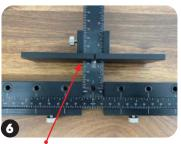
Set Large Stop to measurement from Step 5 and tighten Thumb Screws. (If needed, reverse Large Stop for additional clearance).
