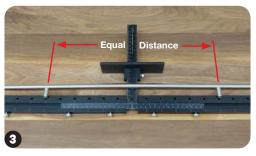
Place hardware on Extension Bars and mark holes to be drilled with tape (if needed, adjust Extension Bars equally left and right until holes align).
