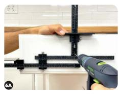
For Knobs: Drill through center bushing.
