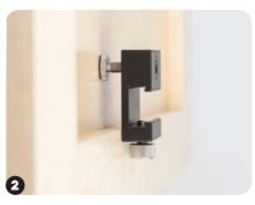
Place Sliding Drill Guide on drawer front with spacer on recessed portion. Adjust until both sit flush.
