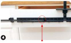
Attach the Extended Ruler to the Extension Bar; set 0 mark on Extended Ruler with marked hole on Extension Bar. (If 0 mark does not work, use another digit and adjust math accordingly).
