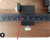
Set Sliding End Stop to measurement from Step 2 and tighten.
