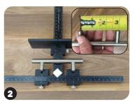
Measure hole centers. Adjust and tighten Sliding Drill Guides. Cover unused bushing with tape or magnet to prevent accidental drilling.
