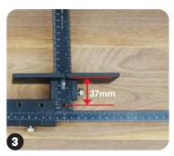
Mount Extension Bar firmly against T-Square. When Large Stop touches Extension Bars, industry standard for shelf pin offset of 37mm is achieved.
