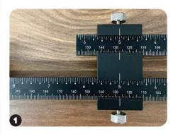
Connect Extended Ruler Attachment and Double Bracket to T-square at 5" mark to extend length of ruler to 16".
