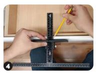
Use half of measurement from Step 3 to mark center on top of drawer.
