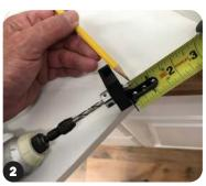
Set Depth Stop Collar to drill depth and tighten. Depth varies depending on screw type and cabinet material.
