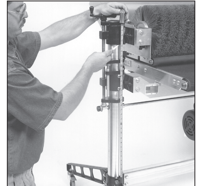
Fig. 18 Comparing brush support casting heights.
