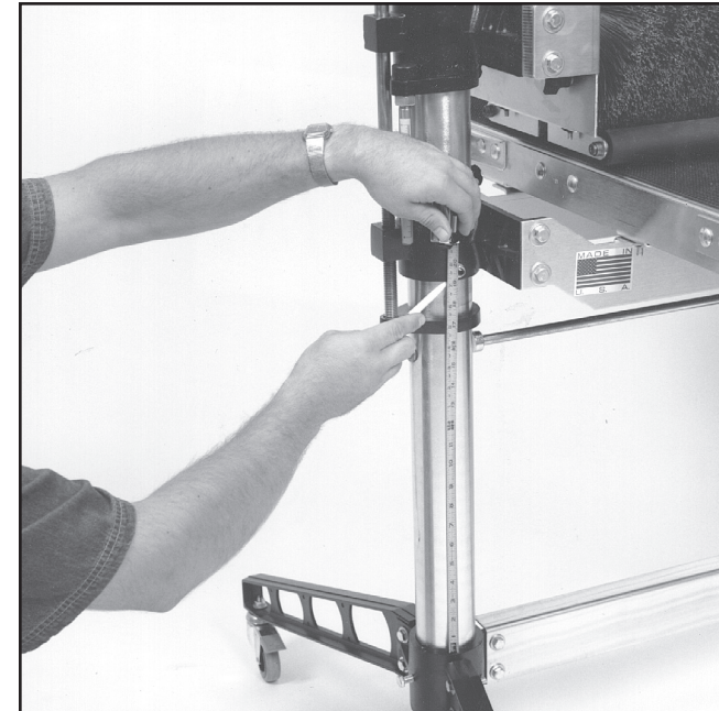
Fig. 17 Adjusting table support castings.
