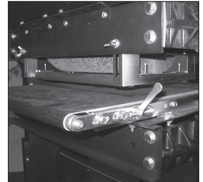
Fig. 21 Tensioning and tracking conveyor belt.
