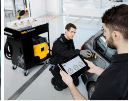
By using the **myMirka®** app you can monitor the vibration level when sanding with Mirka® DEOS.
