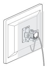
Wire hole allows you to route wires through wire access opening.
