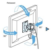
Holds at any angle within 40° up/down tilt Holds at any angle within 180° left/ right swivel
