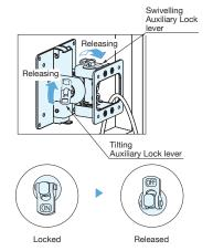
Auxillary locks hold, tilt and swivel to a secure position. Release the lever to adjust the position.
