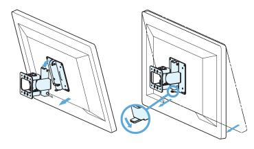
Monitor easily attaches to bracket with slot and click.
