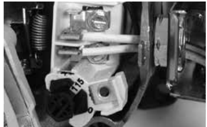
Figure 9 - Voltage set to 115 V, Dial Type
