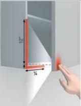
Optimal opening support is achieved if the TIP-ON unit is attached exactly where the handle would be.
