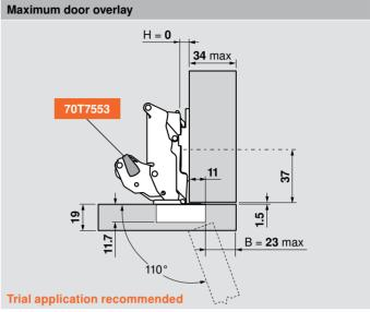
NOTE: Inset application can also be achieved with either a straight-arm hinge with a 18 mm plate or half-cranked hinge with 9 mm plate. Setback of mounting plate would be 38.5 mm + door thickness.
