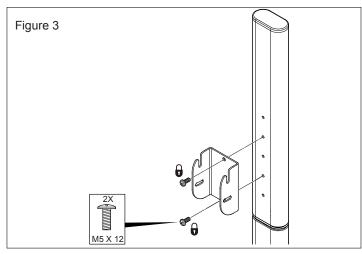
Attach bracket to Ascent with 2 M5 X 12 screws as shown in Figure 3.
