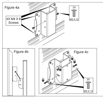
Attach bracket to screen with four M4 X 8 screws. Insert two M5 X 12 screws into the bracket, one on each side (Figure 4A). The M5 X 12 screws support the screen by resting in the slots on the lift bracket (Figure 4B). Insert two M5 X 12 screws into the slotted holes, adjust the tilt angle as desired and secure the bracket position (Figure 4C). This bracket allows screens to vertically tilt up to  $18^{\circ}$ .
