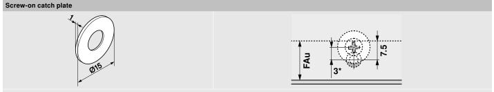
\* We recommend off-setting the positioning of TIP-ON by 3 mm for the screw-on catch plate.
