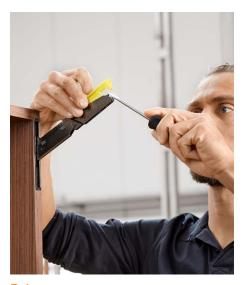
Release the transportation lock over the CLIP mechanism.
