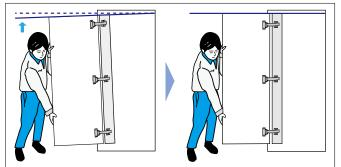
When installing, you can adjust the hanging angle just by lifting up the door.
