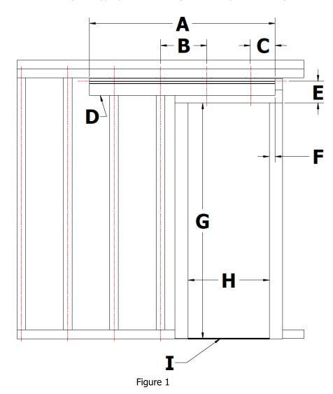
Note: Overlap is the amount of overlap between the Door and Finished Opening when the door is in fully closed position. Ideally, the top, left and right Overlap are equal.
