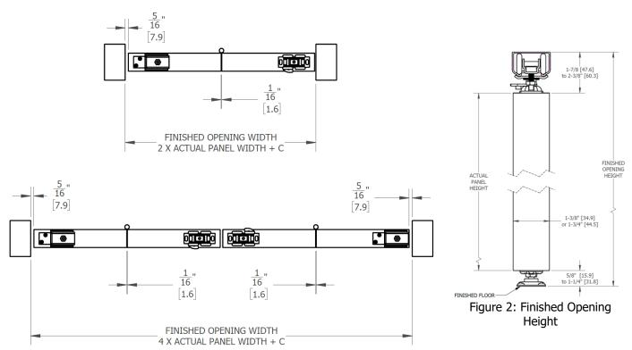
Figure 1: 2-Panel and 4-Panel Finished Opening Width
