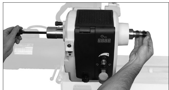
Figure 7-8: removing spur center
