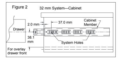
Use only the 32 mm system holes or the wood screw holes located at the tip of the breathing tabs. Do not use any other holes on the cabinet member for mounting (Figure 3).
