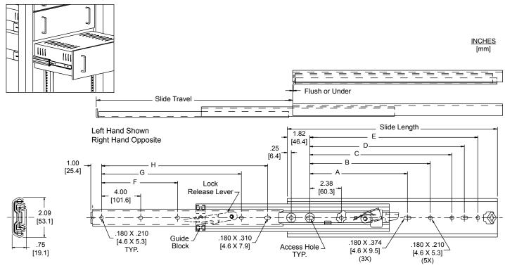
Model 3607 shown (Includes lock-out and lever disconnect)
