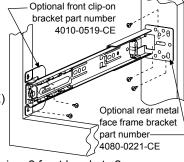
4180-0321-XE. Each kit contains: 2 front brackets 2 rear brackets, and installation instructions. Order 1 kit per pair of slides.
