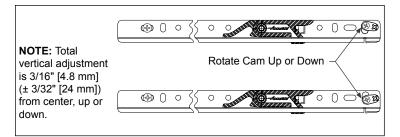
IMPORTANT: After all adjustments are made, secure rail with additional mounting screws.
