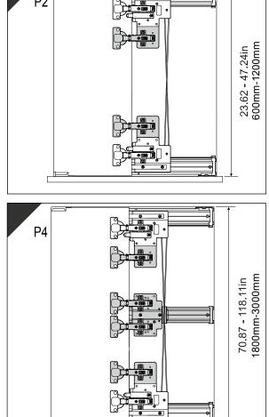
**NOTE**: All fixing positions must be used to achieve maximum load rating.
