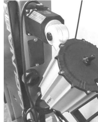
Light fitted in position
