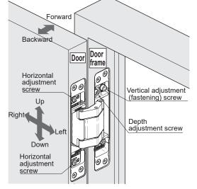
· When adjusting the vertical position or the depth, loosen the screws, then hold the door at the suitable position and re-tighten the screws. Use wedges to support the door. (Tightening torque is  $4.9 \text{ N} \cdot \text{m.}$ )
