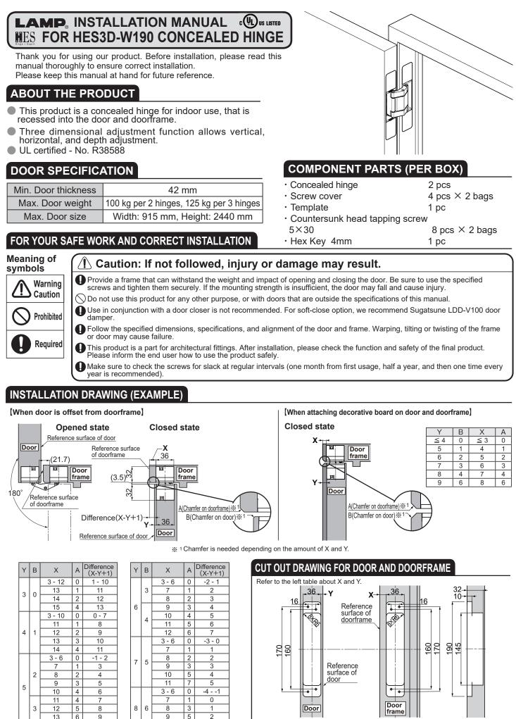
When not using the installation template HES3D-W190-TMP (sold separately) drill pilot holes at the installation screw locations.
