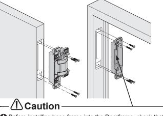
Before installing base frame into the Doorframe, check that it is oriented correctly. If the orientation is incorrect, the door cannot be installed.
