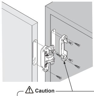
Before installing base frame into the cabinet, check that it is oriented correctly. If the orientation is incorrect, the door cannot be installed.
