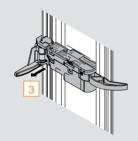
NOTE: For easy replacement mark the current location of the drive unit on the vertical aluminum profile
